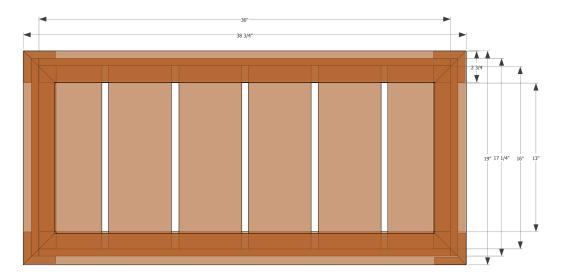
Cut the pickets in half lengthwise and at a 45° angle for the corner pieces.
